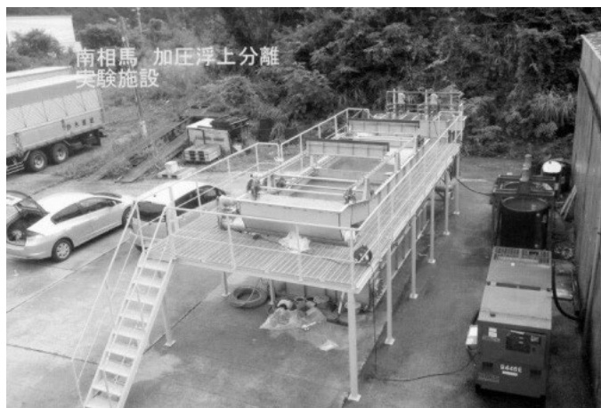
Fig. 1 Floating device for treatment of contaminated site cleaning in Minamisouma test site
