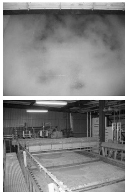
Fig.12 Generated micro bubbles in floating device and floating substance on surface of device
