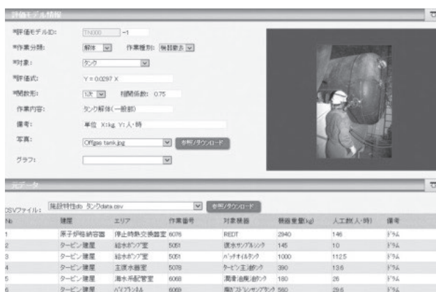
Fig. 10 Example of manpower evaluation model for dismantling tank in JPDR
