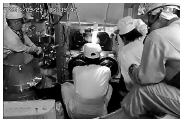
Fig. 16 State of retrieval operation for MARICO-2 test subassembly
